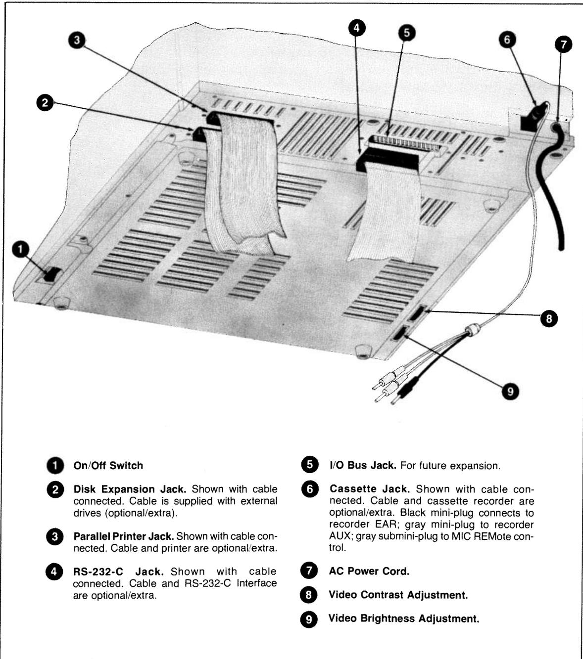
**Figure 1. Connection of peripherals and location of controls.**
