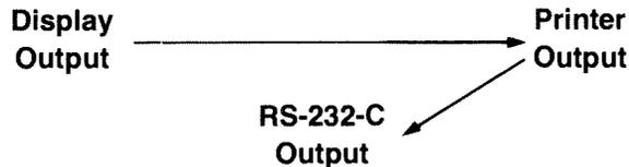
Display output goes to the Printer, and Printer output goes to the RS-232-C. All other I/O routes are unchanged. Note that Display output does **not** get carried forward from the Printer to the RS-232-C. To accomplish the routing pictured above, use this sequence:
