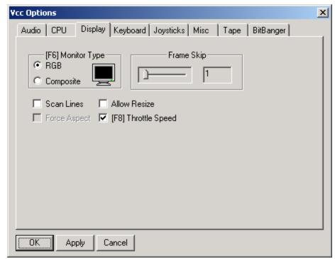
Monitor Type: The Color computer 3 could be attached to 2 types of displays, composite such as a TV or component RGB as in the CM-8 Monitor. Strangely enough each display shows different colors with RGB being the preferred. This allows you to select what "color set" the display will use. This can also be changed via a keyboard shortcut [F6]. See the section on function keys for more information.
