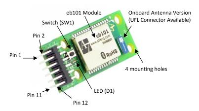
The eb301 features a pin out that provides access to the primary features of the eb101 module.
