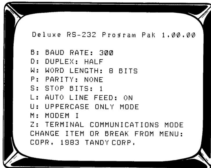
On power-up, the Protocol Menu will always show these settings. If your information service communicates at 300 baud, half-duplex, 8-bit word length, no parity, 1 stop bit, auto line feed ON, uppercase, and is using a Modem I (non-auto dialing modem), you only need to press (BREAK) to begin communications.
