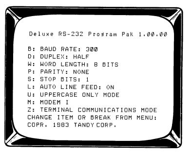
On power-up, the Protocol Menu will always show these settings. If your information service communicates at 300 baud, half-duplex, 8-bit word length, no parity, 1 stop bit, auto line feed ON, uppercase, and is using a Modem I (non-auto dialing modem), you only need to press (BREAK) to begin communications.
