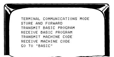
**TERMINAL COMMUNICATIONS MODE** Selecting this mode lets you use your Color Computer as an interactive terminal with a host system. Most information services can be contacted via this mode.
