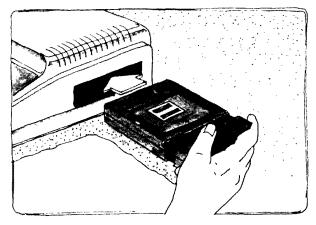
Figure 1. Inserting the RS-232 Program Pak
